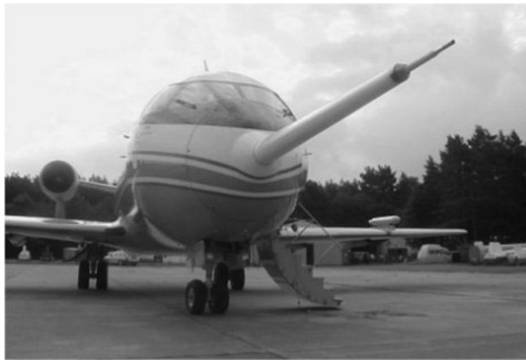
a) Longer noseboom on VFW-614 ATTAS
